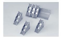
The Magnetic Block holds the target plats of TK1 and TK2. It has corners in various angles so that the reflective surface of the targets creats an angle as close to 90° as possible with the measuring beam.
